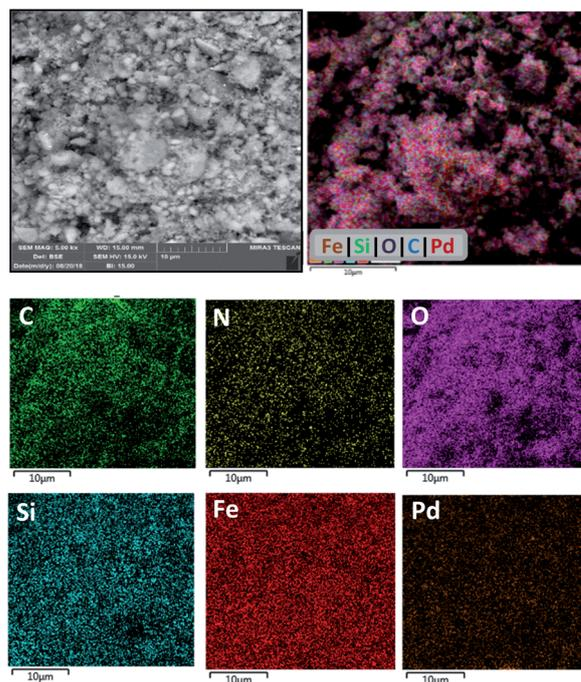
Fig. 5 EDS elemental mappings of the PAMAM  $G_0$ -Pd@ $\gamma$ -Fe<sub>2</sub>O<sub>3</sub> complex.
