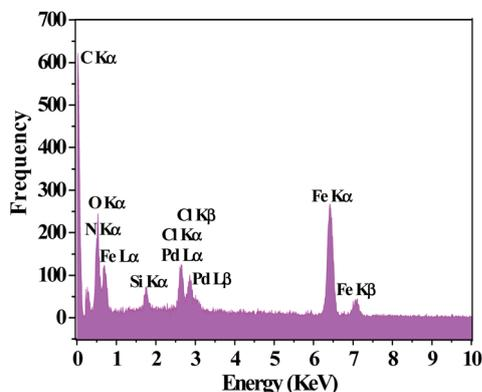
Fig. 4 EDX analysis of the PAMAM  $G_0$ -Pd@ $\gamma$ -Fe<sub>2</sub>O<sub>3</sub> complex.
