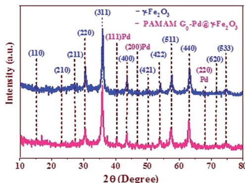
Fig. 2 XRD patterns of  $\gamma$ -Fe<sub>2</sub>O<sub>3</sub>, and PAMAM G<sub>0</sub>-Pd@ $\gamma$ -Fe<sub>2</sub>O<sub>3</sub> complex.
