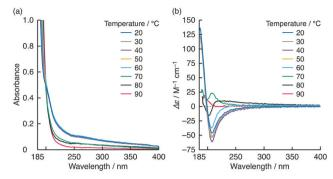
Fig. 5 (a) UV absorption and (b) CD spectra of L-1 (0.2 mM) in water at pH 10 containing NaCl (10 mM) measured at various temperatures (20–90 °C); path length: 0.1 cm. Variations in absorbance at 300 nm and  $\Delta\epsilon$  at 208 nm as a function of temperature are shown in Fig. S16 (ESI†).
