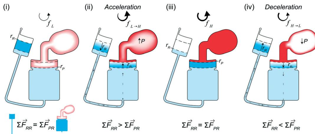
Fig. 2 Stages of CD LR. At a low rotation frequency (i) the forces acting on each column are equal ( $\vec{F}_{RR}$  and  $\vec{F}_{PR}$ ) resulting in the liquid radial positions  $r_R$  and  $r_P$ . Acceleration (ii) increases the centrifugal force, causing liquid to flow from the RR to the PR and the pressure in the GC to increase until the high rotation frequency (iii). Deceleration reverses the process (iv).
