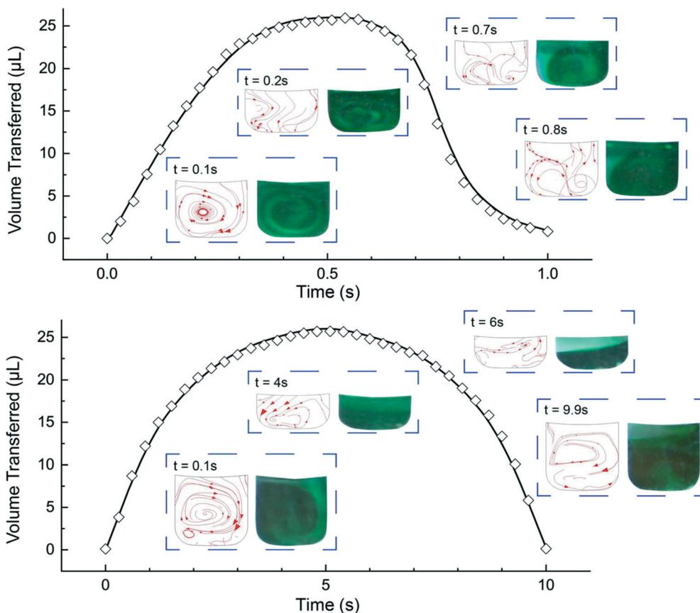
Fig. 4 Comparison between calculated experimental ( $\diamond$ ) and simulated (line) volume transfer during fast LR (top) and slow LR (bottom). Insets compare experimental fluid mixing and simulated streamlines.
