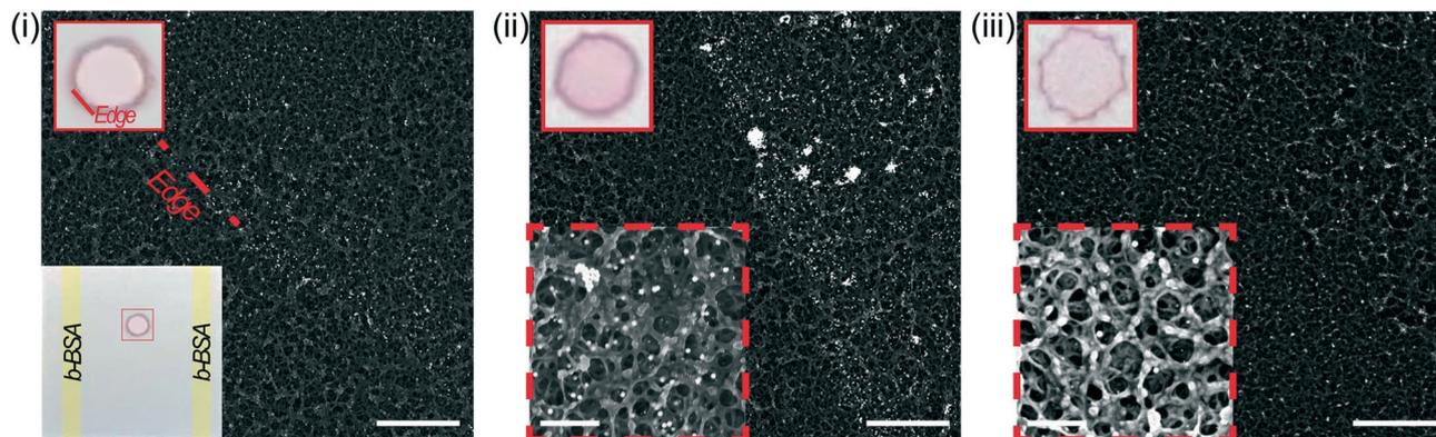
**Fig. 6** SEM images obtained at the edge of the (i) as-printed spots and after a 5 minute incubation on the (ii) benchtop orbital shaker with shear rate  $\sim 10^1 \text{ s}^{-1}$  or (iii) using fast CD LR with shear rate  $\sim 10^3 \text{ s}^{-1}$  (scale bar: 10  $\mu\text{m}$ ; inset scale bar: 2  $\mu\text{m}$ ). Dashed inset at higher magnification and solid inset of regular image illustrating spot deformation cause by fast flow.
