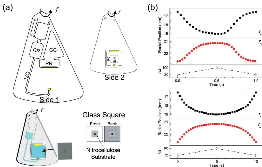
**Fig. 3** (a) A section of the CD used for LR with the primary features labeled (top) and a 3-D illustration of the HI integration with the RC (bot). (b) Measured radial liquid positions during the reciprocation process for a fast LR (top;  $\tau = 1$  s, ramp rate = 160  $\text{Hz s}^{-1}$ ) and slow LR (bot;  $\tau = 10$  s, ramp rate = 16  $\text{Hz s}^{-1}$ ).
