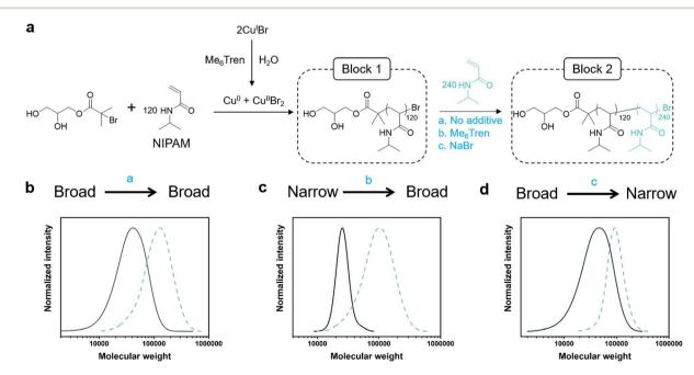
Fig. 2 (a) Synthesis of one-pot PNIPAM-b-PNIPAM with individually tunable blocks via the Cu/L ratio for the first block and either Me<sub>6</sub>Tren or NaBr for the second block. (b) SEC traces for high-to-high, (c) low-to-high, and (d) high-to-low dispersity diblocks.
