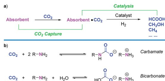
Scheme 1 (a) Schematic CCU concept for CO<sub>2</sub> hydrogenation to C1 products. (b) Reaction pathways for CO<sub>2</sub> absorption with amines under aqueous conditions.
