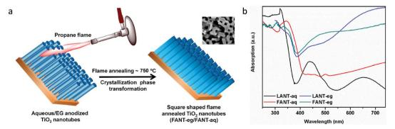
Fig. 15 (a) Synthesis protocol for the generation of oxygen vacancies using propane flame treatment (inset shows TEM image of square-shaped TiO<sub>2</sub> nanotubes after treatment with propane flame) and (b) DRS absorption spectra of LANT-ag, LANT-ag, FANT-ag and FANT-eg samples (reproduced from ref. 66 with permission from Elsevier, copyright 2019).
