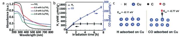
Fig. 25 (a) UV-vis DRS of different samples, (b) time profile for the generation of products, CO and  $H_2$  using 0.5 wt%  $Cu/TiO_2$  photocatalyst, and (c) by use of DFT, calculation of adsorption energy of  $H_2$  and CO on the Cu surface (reproduced from ref. 82 with permission from the Royal Society of Chemistry, copyright 2019).
