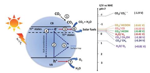
Fig. 1 Schematic illustration of different processes occurring during the photocatalytic conversion of CO<sub>2</sub> into useful products. The absorption of light energy equal to or greater than the bandgap ( $E_q$ ) resulting in excitation of the electrons from the valence band (VB) to the conduction band (CB), leaving behind holes in the VB. The electrons and holes promote the reduction and oxidation of the reactant molecules, respectively.
