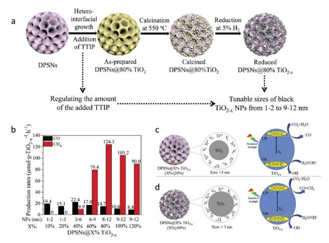
Fig. 9 (a) Synthesis protocol for reduced DPSNs@XX TiO $_{2-x}$  NPs, (b) photocatalytic CO $_2$  conversion using different samples, (c and d) a probable mechanism for the different activity and selectivity of DPSNs@XX TiO $_{2-x}$  NPs with the varied particle size of black TiO $_{2-x}$  NPs for CO $_2$  conversion (reproduced from ref. 52 with permission from Elsevier, copyright 2019).
