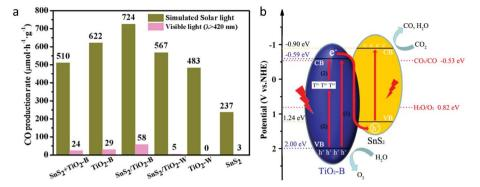
Fig. 28 (a) Comparison of the yield of CO produced by photocatalytic  $CO_2$  conversion using  $SnS_2/TiO_2$ –B under simulated solar light and visible light and (b) schematic for the Z-scheme mechanism of separation of photogenerated charge carriers (reproduced from ref. 87 with permission from MDPI, copyright 2019).
