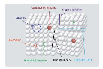
Fig. 2 Schematic of the different types of defects present in the  ${\rm TiO_2}$  crystal.
