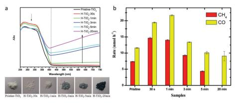
Fig. 14 (a) DRS spectra and the photograph of the samples with increasing plasma treatment time and (b) photocatalytic  $CO_2$  conversion using hydrogenated samples under solar light illumination (reproduced from ref. 62 with permission from the Royal Society of Chemistry, copyright 2014).
