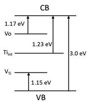
Fig. 5 Energy levels formed due to the presence of defects such as oxygen vacancy, titanium vacancy and titanium interstitial within the bandgap of reduced rutile  $\text{TiO}_{2-x}$ . Energy levels were taken from ref. 46
