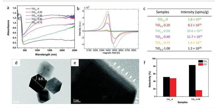
Fig. 20 (a) DRS absorption spectra, (b) EPR spectra and (c) the spin intensity of reduced  $TiO_2$  samples, (d) HRTEM image of  $TiO_{2-x}$ -0.50, (e) disordered layers on the surface of  $TiO_{2-x}$  marked with white color arrows and (f) selectivity for  $CH_4$  and CO generation using  $TiO_{2-x}$ -0 and  $TiO_{2-x}$ -0.50 in the absence of the cocatalyst and under simulated solar light (reproduced from ref. 74 with permission from the Royal Society of Chemistry, copyright 2017).
