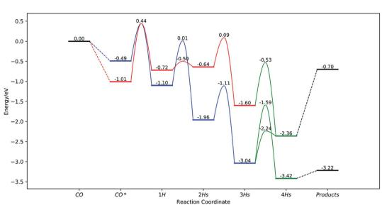
Fig. 7 Overall potential energy surface from CO to CH<sub>4</sub>. Black, red, blue, and green bars and curves represent a desorption state, the most favorable pathway for CO(A), the most favorable pathway for CO(B) and pathways after merged, respectively (reproduced from ref. 49 with permission from the American Chemical Society, copyright 2019).
