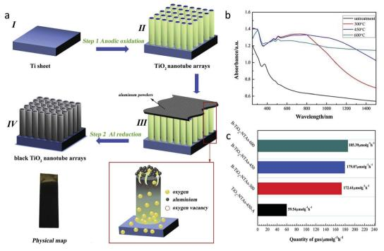
Fig. 17 (a) Schematic of synthesis procedure for the black  $TiO_2$  nanotube array, (b) UV-visible DRS spectra of the sample annealed at different temperatures and (c) photocatalytic  $CO_2$  conversion using different samples under visible light illumination (reproduced from ref. 70 with permission from Elsevier, copyright 2020).
