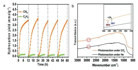
Fig. 13 (a) Stability evaluation of Cu-Pt modified blue titania for photocatalytic  $CO_2$  conversion, (b) FTIR analysis of the sample after photocatalytic reaction carried out in the presence of  $CO_2$  and He gas (reproduced from ref. 61 with permission from the Royal Society of Chemistry, copyright 2019).
