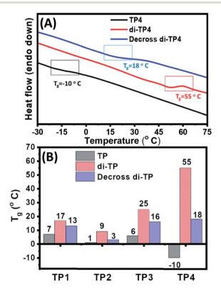
Fig. 5 (A) Representative DSC traces showing effect of photodimerization on the glass transition temperature of the polymer films (20 mg mL<sup>-1</sup>) of native TP4, crosslinked di-TP4 and decrosslinked di-TP4. (B) The glass transition temperatures for TP1–TP4 polymers in native, crosslinked and decrosslinked forms.
