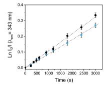
Fig. 7 First-order plots for the oxidation of Trp (20 mM) photosensitized by the PEDOT- $C_{60}$  surface ( $\blacksquare$ ) and fullerene  $C_{60}$  ( $\blacksquare$ ) in DMF solution,  $\lambda_{irr} = 455-800$  nm.
