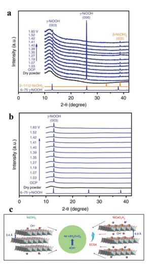
Fig. 5 (a and b) Operando XRD patterns collected on (a) Ni(OH)<sub>2</sub>/NF and (b) NiCeO<sub>x</sub>H<sub>y</sub> /NF electrodes at different potentials. (c) The OER proceeds more favourably on NiCeO<sub>x</sub>H<sub>v</sub> with larger interlamellar spacing and higher ECSA relative to Ni(OH)<sub>2</sub>.59
