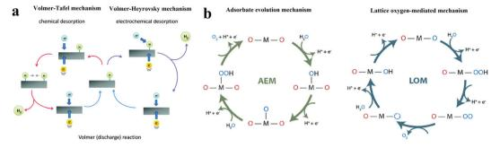
Fig. 1 (a) The schematic of electrocatalytic turn-over of hydrogen evolution on the surface of an electrode. 21 (b) The adsorbate evolution mechanism (AEM) and lattice oxygen mediated mechanism (LOM) of oxygen evolution turnover on the surface of catalyst.<sup>23</sup>
