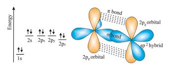
Fig. 11 Scheme of electron configuration and the corresponding sp<sup>2</sup> hybrids and  $\boldsymbol{\pi}$  orbitals of the carbon double bond
