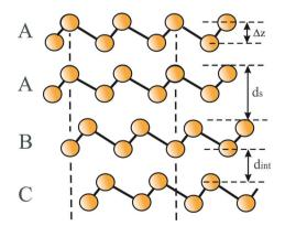
Fig. 15 The stacking orders AA, AB, and AC of bilayers of buckled hexagonal monolayers. This figure defines the buckling effect  $\Delta z$ , the interlayer spacing ds, and the distance between adjacent layers  $d_{\text{int}}$ .
