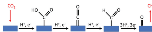
Fig. 27 A postulated mechanism of methane formation from the electrochemical reduction of CO 2 . Adapted with permission from ref. 199. Copyright (2015) American Chemical Society.
