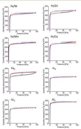
Fig. 5 Nitrogen Isotherms at 77 K before (red) and after (blue) 100 hour thermal activation. In the Fe/Ni, Fe/Zn, Fe/Mn, Fe/Co, Fe<sub>3</sub>, clusters a hysteresis loop is observable indicating mesopore formation. Samples for In<sub>3</sub>, Sc<sub>3</sub>, and Al<sub>3</sub> do not have mesopore formation.
