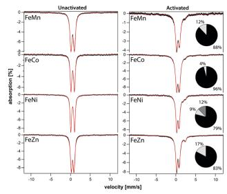
Fig. 3 Mössbauer spectra of unactivated (left) and activated (right) mixedmetal MOFs. Spectra were collected at 5 K and 0.05 T with the applied field parallel to the gamma radiation. Black hashmarks are data; red lines are simulations. Black column inset quantifies the dominant quadrupole doublet and any minor amount of magnetic material extending from the baseline. The light grey columns indicate the percentage of Fe<sup>II</sup> sites.
