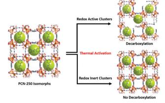
Fig. 7 The findings of the study indicate the dependence of thermally induced decarboxylation on the redox activity of the clusters in the isomorphs of PCN-250
