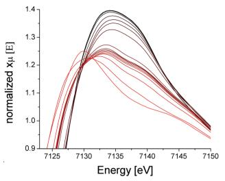
Fig. 4 XAS spectra of PCN-250 (Fe\_3) in the range of 23  $^{\circ}\text{C}$  (black) to 450  $^{\circ}\text{C}$  (red).
