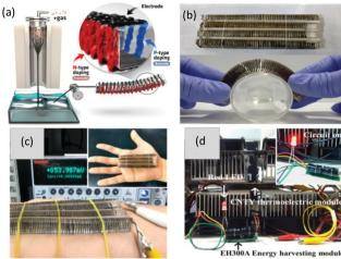
Fig. 6 (a) Fabrication process of the CNTY and flexible TE device. (b) Picture showing the flexibility of the fabricated TEG. (c) Output voltage obtained from the TEG using body heat. (d) Image of a red LED powered using the flexible TEG at  $\Delta T$  = 50 K. Reprinted with permission from ref. 20 (J. Choi, Y. Jung, S. J. Yang, J. Y. Oh, J. Oh, K. Jo, J. G. Son, S. E. Moon, C. R. Park, H. Kim, 11 (2017) 7608-7614). Copyright (2017) ACS Publications.
