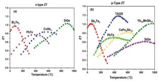
Fig. 3 ZT values of different materials in different temperature ranges (a) for n-type and (b) for p-type materials. Commercial alloys of bismuth and antimony tellurides from Marlow industries (unpublished data); types of doped PbTe;7 skutterudite alloys of CoSb3 and CeFe4Sb12 from JPL, Caltech (unpublished data); TAGS;8 doped SiGe;9 Yb14MnSb11;10 Redrawn from ref. 8
