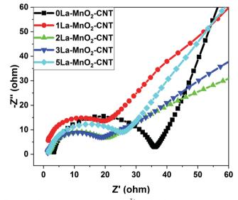
Fig. 11 EIS spectra of undoped and La<sup>3+</sup>:MnO<sub>2</sub>-CNT nanohybrids.
