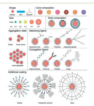
Fig. 2 The different components/shapes of those components in QDs which generate different QDs. Due to the number of different components, it means that they differ in shape/size/properties.<sup>20</sup>
