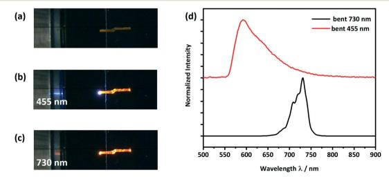
Fig. 8 Optical microscope images of (a) the bent crystal placed on a silicon wafer with a 3  $\mu$ m thick SiO<sub>2</sub> layer, (b) showing light with a wavelength of 455 nm being coupled at the left end of the crystal and (c) showing light with a wavelength of 730 nm being coupled at the left end of the crystal; (d) detected PL-spectra at the right end of the crystal.
