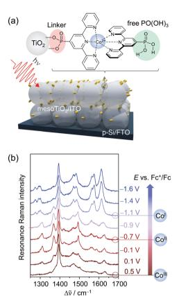
Fig. 7 (a) Phosphonic acid modified Co bisterpyridine adsorbed on mesoporous TiO<sub>2</sub> or ITO (mesoTiO<sub>2</sub>/mesoITO). (b) EC-RR spectra revealing the reduction of adsorbed CotpyP on mesoITO from Co<sup>III</sup> to Co<sup>II</sup> to Co<sup>II</sup> in the potential range from 0.5  $V_{Fc^+/Fc}$  to  $-1.6 V_{Fc^+/Fc}$  (514 nm excitation, acetonitrile with 0.1 M TBABF<sub>4</sub>). Graph redrawn from ref. 71.
