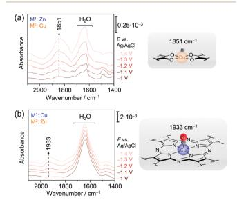
Fig. 10 EC-SEIRA difference spectra of CNT-Pc $|Zn-O_8|$ Cu (a) and CNT-Pc|Cu- $O_8$ |Zn (b) under CO<sub>2</sub>RR conditions (0.1 M KHCO<sub>3</sub>). The rising band at  $1851\,\text{cm}^{-1}$  reflects the formation of the hydride species H-CuO<sub>4</sub> in the CuO<sub>4</sub> motif. In the presence of a CuN<sub>4</sub> structure motif, binding of a CO to CuN<sub>4</sub> is observed by a redshifted  $\nu$ (CO) mode at 1933 cm<sup>-1</sup>. Graphs redrawn from ref. 78.
