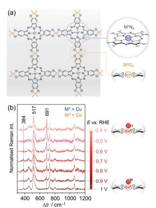
Fig. 9 (a) Structure of bimetallic 2D c-MOFs consisting of phthalocyanine units (blue circle) linked via oxygen nodes (orange circle). M<sup>1</sup>N<sub>4</sub> and M<sup>2</sup>O<sub>4</sub> denote the two metal centres in the respective coordination environment. (b) EC-Raman spectra of CNT-Pc|Cu-O<sub>8</sub>|Co during ORR (413 nm excitation, 0.1 M KOH) suggesting the formation of the  $Co^{III}$ – $O_x$  intermediate at 691 cm<sup>-1</sup>. Scheme and graph redrawn from ref. 79.
