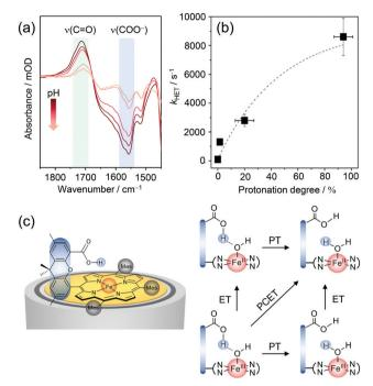
Fig. 4 (a) pH dependent SEIRA spectra showing the protonation of the carboxylic acid hanging group upon lowering the pH. (b) Correlation between the rate of porphyrin reduction ( $k_{\rm HET}$ ) and protonation grade of the hanging group. (c) Proposed scheme for proton-coupled electron transfer (PCET) in Fe–Hangman complexes with a protonated carboxylic acid hanging group. Graphs and scheme redrawn from ref. 57.
