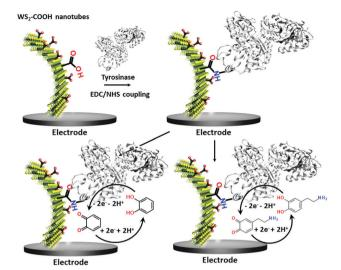
Scheme 1 Sketch of the functionalization of WS<sub>2</sub> modified glassy carbon electrodes with the enzyme tyrosinase via a standard EDC/NHS coupling reaction. These modified bioelectrodes served in the detection of catechol (bottom left) and dopamine (bottom right) at  $-0.2 \text{ V vs. Ag}^+/\text{Ag}$
