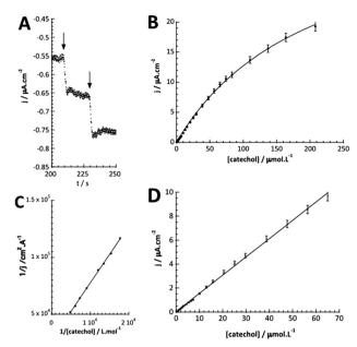
Fig. 4 (A) Chronoamperometric response of the GC/WS $_2$ -COOH/tyrosinase electrode ( $E=-0.2~V~vs.~SCE;~0.1~mol~L^{-1}~PBS;~pH~7.4$ ) upon successive increase of catechol concentration from 0.3  $\mu$ mol L $^{-1}$  to 220  $\mu$ mol L $^{-1}$ . (B) Plot of the current density vs.~ catechol concentration on tyrosinase/WS $_2$ -COOH/GCE. (C) Lineweaver–Burk plot of the corresponding data. (D) Plot of the linear part of the current density vs.~ increasing catechol concentrations.
