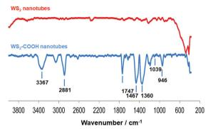
Fig. 6 IR spectra of WS<sub>2</sub> nanotubes before (top) and after (below) carboxylation.
