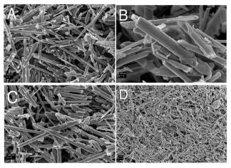
SEM images of (A and B) as synthesized WS2-COOH powder at magnifications of (A) ×20 000 and (B) ×50 000. SEM images of (C and D) thin films of WS<sub>2</sub>-COOH nanotubes at magnifications of (C) ×20 000 and (D) ×5000.
