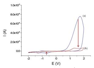
Fig. 3 Voltammograms obtained in  $CH_3CN + 0.1 \text{ mol L}^{-1} \text{ TBAP}$ ; first cycle (a) and second cycle (b) with the GCE/WS<sub>2</sub>-COOH modified electrode between -2.0 and +2.0 V vs.  $Ag^+/Ag$ ; scan rate: 100 mV s<sup>-1</sup>.
