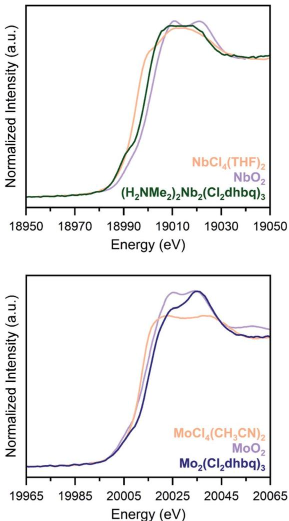
Fig. 2 K-edge X-ray absorption spectra for **1-Nb** (top) and **2-Mo** (bottom), along with tetravalent metal oxides (orange) and molecular chloride complexes (purple), as reference compounds. Both frameworks display pre-edge features which are indicative of a trigonal prismatic geometry. Data for  $\text{NbO}_2$  and  $\text{MoO}_2$  are taken from ref. 34 and 53.
