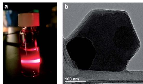
Fig. 4 (a) Photograph of scattered 635 nm light from a suspension of **2-Mo** in DMF demonstrating the Tyndall effect. (b) TEM image of a few-layer nanosheet of **2-Mo**. Additional images are shown in Fig. S18<sup>†</sup>
