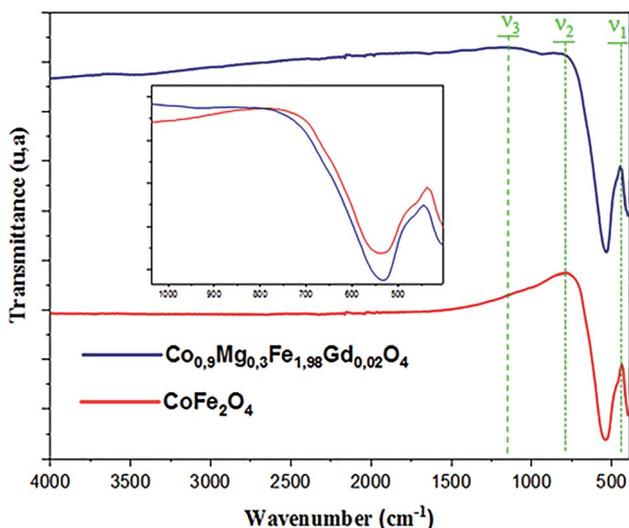
Fig. 4 FTIR spectra of samples  $\text{Co}_{0.7}\text{Mg}_{0.3}\text{Fe}_{1.98}\text{Gd}_{0.02}\text{O}_4$  and  $\text{CoFe}_2\text{O}_4$ .
