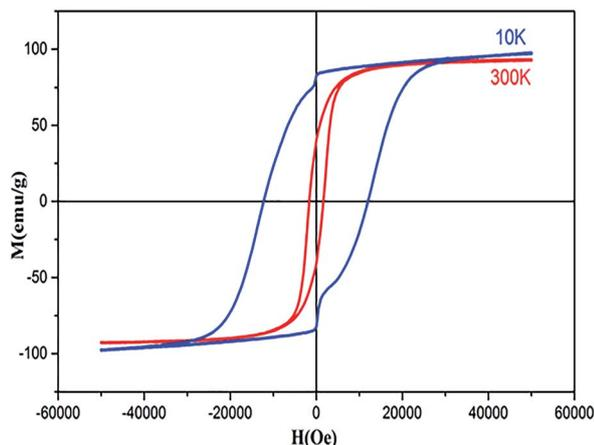
Fig. 7 Hysteresis loops of sample  $\text{Co}_{0.7}\text{Mg}_{0.3}\text{Fe}_{1.98}\text{Gd}_{0.02}\text{O}_4$ .
