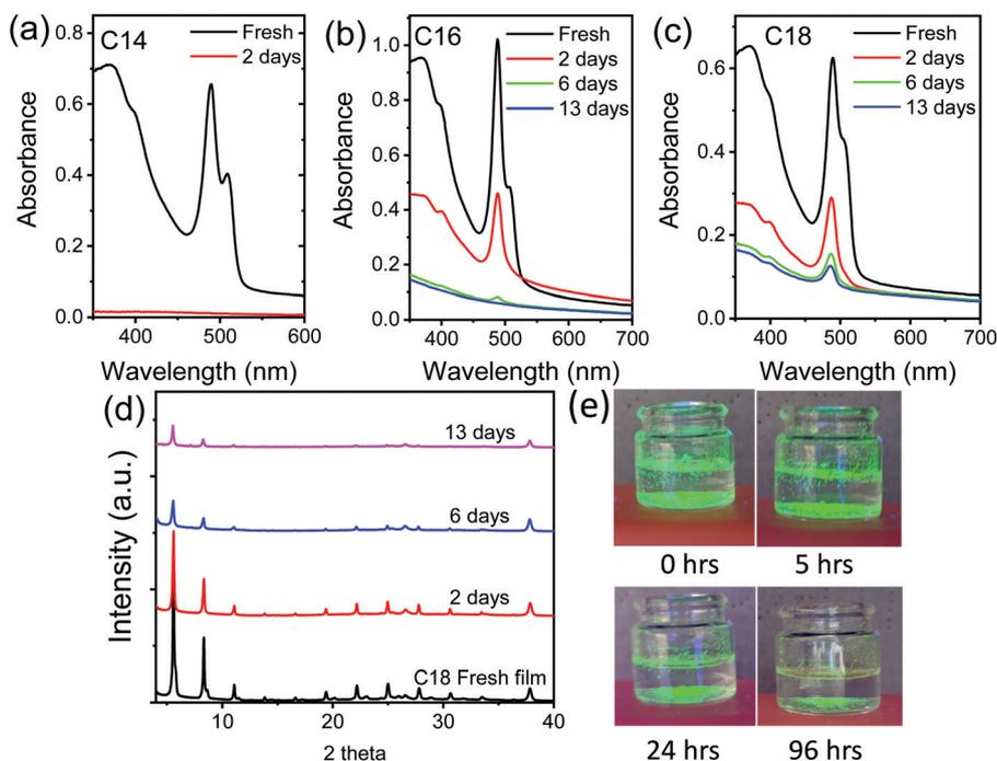
**Fig. 4** Absorption spectra of (a)  $(C_{14}H_{29}NH_3)_2PbI_4$ , (b)  $(C_{16}H_{33}NH_3)_2PbI_4$  and (c)  $(C_{18}H_{37}NH_3)_2PbI_4$  2D perovskites thin films immersed in water. (d) XRD pattern of  $(C_{18}H_{37}NH_3)_2PbI_4$  thin film immersed in water and (e) bright green light emission from the  $(C_{14}H_{29}NH_3)_2PbI_4$  powder sample immersed in water and kept under continuous UV light (365 nm) illumination.
