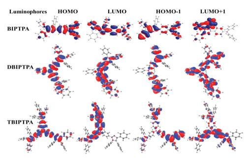
Electron density outlines of the frontier molecular orbitals (FMOs) of the luminophores
