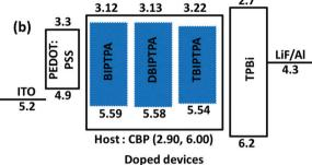
Fig. 8 Schematic representation of the energy levels of the solution-processed OLEDs composed of deep-blue BIPTPA, DBIPTPA and TBIPTPA emitters (a) undoped and (b) doped in CBP host devices.
