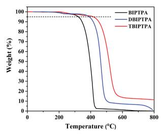
Fig. 1 Thermogravimetric curves of the luminophores.
