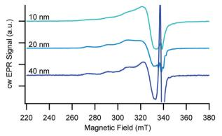
Fig. 2 Continuous wave X-band EPR spectra of  $\bf 3$  in the Cu(II) oxidation state immobilized on 10, 20, and 40 nm AAO recorded at T=20 K.
