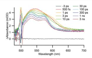
Fig. 4 Ultrafast transient absorption spectra of  $\bf 3$  on 10 nm AAO in deaerated CH<sub>2</sub>Cl<sub>2</sub>. Excitation at 500 nm, time delay noted in legend.
