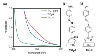
Fig. 3 (a) UV-vis spectra comparing the solid-state absorption spectra of TiO<sub>2</sub>-Bare, TiO<sub>2</sub>-2 and TiO<sub>2</sub>-3. Structures of (b) TiO<sub>2</sub>-2 and (c) TiO<sub>2</sub>-3.
