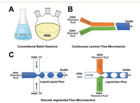
Fig. 1 Schematic illustrations showing examples of different types of reactors: (A) conventional batch reactors; (B) continuous laminar flow microreactors; and (C) discrete segmented flow microreactors.
