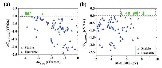
Fig. 5 The dependence of the reaction energy  $\Delta G_{\text{LLZOM-Li}}$  of Li|LLZOM interface on (a)  $\Delta H_{f,x+y}$  and (b) M-O bond dissociation energy. The dotted boxes represent the most appropriate range for each feature.
