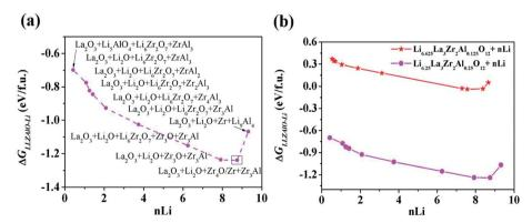
Fig. 2 The thermodynamic stability of LLZOAl when it reacts with Li. (a) The reaction paths and product phases along the dashed lines are marked, and the lowest reaction energy is marked with a square. (b) The reaction energy of the Li|LLZOAI interface vs. the doping concentration.
