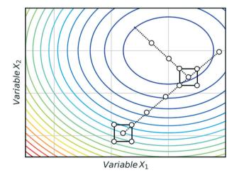
Fig. 6 A steepest descent method minimisation, where an initial point and 2<sup>k</sup> orthogonal design are performed, followed by further experiments along the trajectory of highest gradient towards the optimum. Minima (blue), maxima (red).
