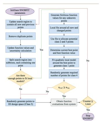
Fig. 7 Flow diagram for a call of the SNOBFIT algorithm.  $n_{\text{eval}}$  is the current number of points for the following iteration SNOBFIT has generated.  $n_{\text{req}}$  is the required number of points to be generated for each call of the algorithm, this is set by the user.
