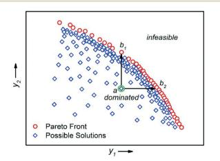
Fig. 9 An example of a multi-objective optimisation with two competing maximisation performance criteria  $y_1$  and  $y_2$ . The Pareto front is the series of non-dominated solutions,  $y(x^*)$ . Solution a is dominated by all solutions between  $b_1$  and  $b_2$ .
