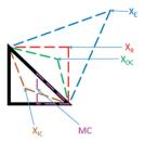
Fig. 2 The different geometric transformations of the Nelder-Mead simplex: inside contraction (X<sub>IC</sub>), multiple contraction (MC), outside contraction ( $X_{OC}$ ), reflection ( $X_R$ ) and expansion ( $X_E$ ).
