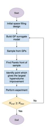
Fig. 12 Flow diagram for the TSEMO algorithm.  $N_{\text{eval}}$  is the current number of evaluations and  $N_{\rm max}$  is the maximum number of evaluations.
