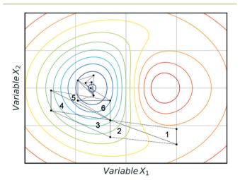
Fig. 3 An example of a two-variable design space with arbitrary variables and a mapped response surface, showing how NMSIM converges on the minimum. Minima (blue), maxima (red).
