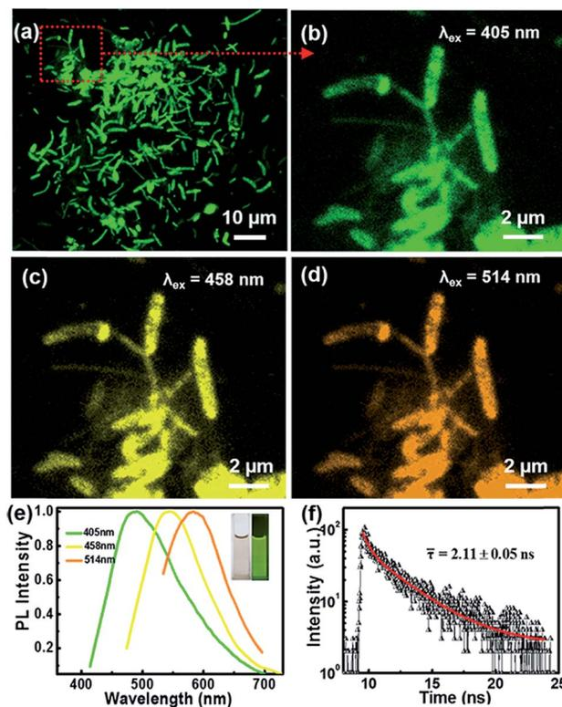
Fig. 3 (a) LCFM image of the full view of CNBs ( $\lambda_{\text{ex}} = 405\text{ nm}$ ). The enlarged LCFM images of CNBs were obtained under excitation at (b) 405 nm, (c) 458 nm and (d) 514 nm. (e) PL emission spectra of CNB aqueous solution. Inset: photos of the aqueous solution under sunlight and a UV lamp (365 nm). (f) PL decay lifetime spectrum and fitting curve (red line) of CNBs ( $\lambda_{\text{ex}} = 405\text{ nm}$ ).
