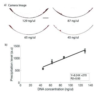
**Fig. 4** DNA quantification on the LOD platform. CMOS sensor generated precipitate images of a known amount of PCR product. a) Four different concentrations imaged with a CMOS camera with 45 ng  $\mu l^{-1}$  being the lowest detectable concentration. Scale bar: 1 mm. b) Calibration curve of the precipitation level *versus* known DNA concentration.
