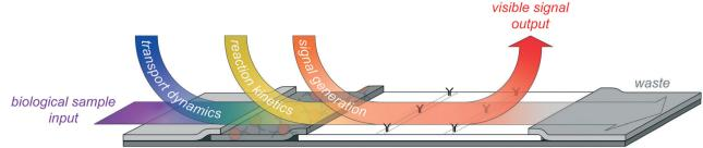
Fig. 2 Illustration of the overlapping dynamics in an LFA system, by which its physical (transport dynamics), chemical (reaction kinetics), and optical (signal generation) properties are interconnected in a highly complex, time-dependent fashion. State-of-the-art improvements to LFA sensitivity must accommodate these interconnected system dynamics.
