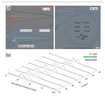
Fig. 8 (a) Performance of the chip with R 0.5 mm and 10  $\times$  20  $\mu$ m (H  $\times$ W) with bacteria at 80 bar (120 μL min<sup>-1</sup>); Escherichia coli, Salmonella and Klebsiella. (b) Intensity profiles of the bacteria at 20 to 80 bar (30 to 120 µL min<sup>-1</sup>). In the normalized channel, width 0 represents the inner wall.
