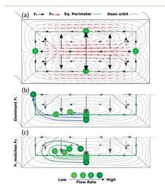
Fig. 6 (a) Simplified, conceptual version of the map of  $F_{\perp}$  for straight channels (omitting the strong wall force that repels particles towards the equilibrium perimeter) with an overimposed secondary flow at 50  $\mu$ L min<sup>-1</sup>. (b) Migration of particles in a scenario where  $F_L$  dominates and (c) where  $F_L$  matches  $F_D$ .
