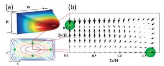
Fig. 1 (a) 3D flow profile in a straight microchannel (aspect ratio W/H = 2) and its representation in 2D with isovelocity curves showing the equilibrium positions for particles with a/H = 0.1. (b) Map of the net force acting on such particles at Re = 100, based on the results of Chao Liu *et al.*<sup>24</sup>
