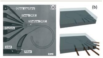
Fig. 2 (a) Microfluidic chip consisting of two curves with 0.5 mm in radius (R); 10  $\mu$ m in depth (H) and 20  $\mu$ m in width (W) connected by a small turn (30  $\mu$ m in R). (b) Sketch of the fabrication.
