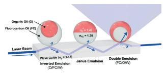
Fig. 1 Conceptual sketch of the modular sensing approach consisting of dynamic complex emulsions in three different morphologies on top of a waveguide-based sensing device. Beginning on the left, total internal reflection (TIR) is observed for inverted and Janus emulsions. Upon transition to a double emulsion with the higher index organic phase on the outside, the laser light is out-coupled from the waveguide, thereby increasing light intensity measured above the waveguide.
