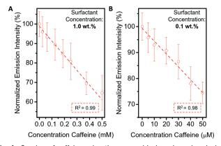
Fig. 4 Sensing of caffeine using the waveguide-based sensing device. The sensitivity can be fine-tuned through variations of the overall surfactant concentration in solution. Emission intensity decrease as a function of caffeine concentration for emulsions in a (A) 1.0 wt% and (B) 0.1 wt% surfactant solution (ratio of  $C_{10}P$ : Zonyl surfactants: 95:5).
