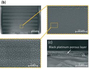
Fig. 2 (a) Optical image of a microfluidic channel with a gold electrode that has an increasing area from bottom to top electrodeposited with platinum black. (b) Scanning electron microscopy (SEM) images of the electrodeposited areas and (c) the thickness of the platinum black layer.
