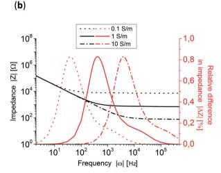
Fig. 3 (a) Schematic of the FEM design used to simulate the increasing electrodeposited area system. On both sides 2 layers of SU-8 are simulated and 2 layers of glass at the top and bottom of the channel are simulated but not shown. (b) Three simulated Bode plots and difference in relative impedance with conductivities of 0.1, 1 and 10 S m $^{-1}$  of two polystyrene particles 83  $\mu m$  in diameter at the top and bottom positions in the x-direction in the microfluidic channel.
