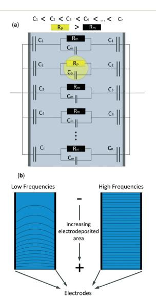
Fig. 1 (a) Simplified electrical equivalent circuit of a parallel electrode array with an increasing electrodeposited area at both electrodes and a particle placed in the cell. (b) Current density simulation of a two platinum electrodes with an increasing electrodeposited area at lower and higher frequencies.
