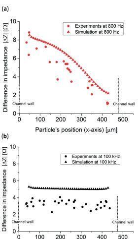
Fig. 6 Experimental results and simulation of the impedance difference obtained from 83  $\mu m$  polystyrene particles at (a) 800 Hz and (b) 100 kHz.
