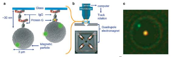
Fig. 8 Study of single protein molecules using rotating MPs in an eMTT, by A. van Reenen et al.<sup>70</sup> (a) MPs are bound to a glass substrate by via a molecular complex. (b) Inside a fluid cell, the particles are actuated by a rotating magnetic field generated by a quadrupole electromagnet. (c) The particle orientation is visualized by means of attached small green fluorescent spheres. The bright spot in the center of the particle is caused by the excitation light.
