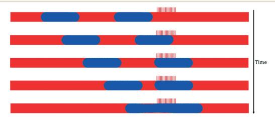
Fig. 3 Time-lapse snapshots of the phase distribution in a capillary microseparator during normal operation ( $\Delta P_{\text{outlet}} = 1820 \text{ Pa}$ ). Here, toluene is the wetting phase (red) and water is the non-wetting phase (blue).  $\Delta t = 0.15 \text{ s}$ .
