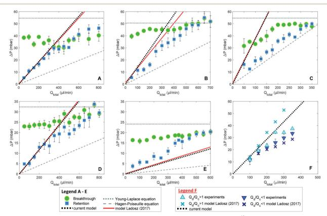
Fig. 8 Comparison of model predictions in this work with the results of Ładosz and Rudolf von Rohr; 48 A-F: flow rate ratio equal to one, five capillary geometries were tested, with capillary dimensions denoted in µm as width-length: A: 10-250; B: 10-500; C: 10-1000; D: 20-1000; E: 30-1000; F: varied flow rate ratio experiments using separator 10-500, only retention bound shown.
