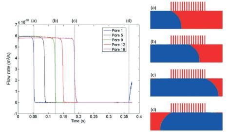
Fig. 6 Real-time flow rates through different capillary pores obtained from CFD simulation. In this case, a segment of non-wetting phase moved through the capillary region without entering into the pores, corresponding to the normal operation regime. Pore 1 referred to the leftmost capillary channel, while pore 16 was the rightmost. Only the top half of the channel was simulated (with symmetric boundary condition on the bottom) to reduce computation time.
