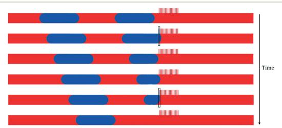
Fig. 4 Time-lapse snapshots of the phase distribution in a capillary microseparator during breakthrough ( $\Delta P_{\text{outlet}} = 3640 \text{ Pa}$ ). Here, toluene is the wetting phase (red) and water is the non-wetting phase (blue).  $\Delta t = 0.05$  s. The black box highlights the capillaries through which breakthrough occurred.
