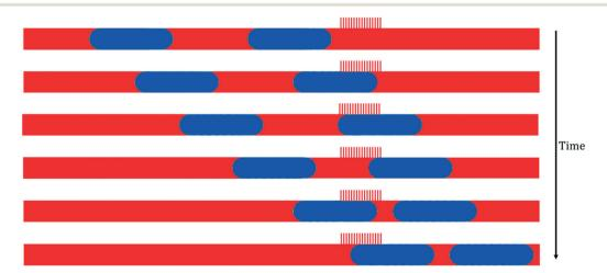
Fig. 5 Liquid-liquid phase distribution in a capillary microseparator capturing the retention phenomenon (ΔP<sub>outlet</sub> = 30 Pa). Here, toluene is the wetting phase (red) and water is the non-wetting phase (blue).  $\Delta t = 0.15$  s.
