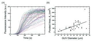
Fig. 6 High-throughput membrane transport measurements using a single device. (A) Fluorescence traces of calcein influx from 66 GUVs pre-incubated with  $\alpha$ -HL membrane pores. (B) Total porated area plotted against GUV diameter. The straight line fit is a guide to the eye.
