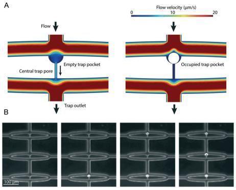
Fig. 2 Overview of flow dynamics and operation of the single-cell trap. (A) FEM simulation of the flow velocities ( $\mu$ m s<sup>-1</sup>; color-coded) in and around the hydrodynamic single-cell trap with an empty (left) or occupied (right) trap pocket. Occupation of the trap prevents fluid flow through the centrally located trap pore. (B) Image sequence showing the trapping of three individual cells in the three serially connected traps.
