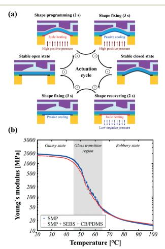
Fig. 2 Working principle of our SMP valves. (a) Schematic illustration of the complete valve actuation cycle (open → closed → open). By combining pneumatic pressure and Joule heating, each valve can be cyclically open and closed. (b) Measured Young's modulus versus temperature for the SMP material used as a single thin layer and in the tri-layer.
