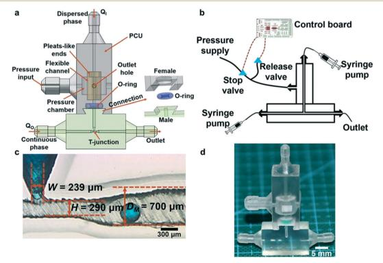
Fig. 9 (a) Schematic of the pneumatic device for droplet generation. (b) Schematic of the experimental setup. (c) Photograph showing T-junction channel. (d) A printed pneumatic device for emulsion generation. Reproduced from ref. 76 with permission.
