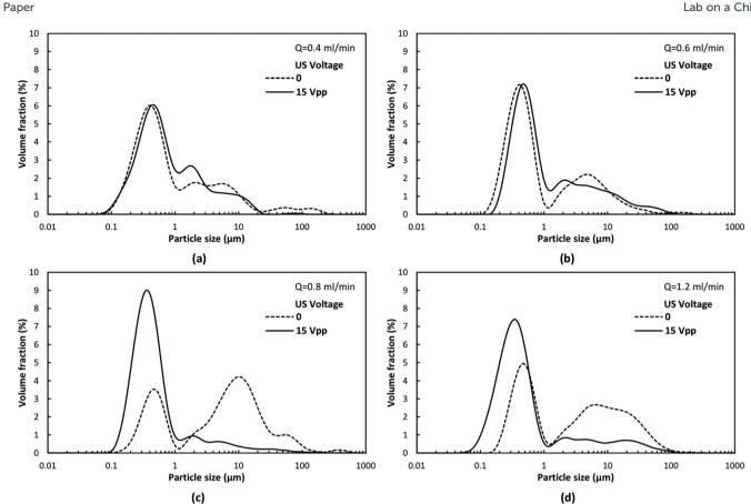
Fig. 8 Effect of US on the CaCO<sub>3</sub> particle size distribution at different flow rates.
