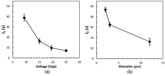
Fig. 6 Influence of (a) applied US voltage and (b) mean particle size on the focusing time t<sub>F</sub>. The particle size in Fig. 6(a) is 12 μm. The applied voltage in Fig. 6(b) is 15 Vpp.
