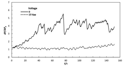
Fig. 7 Normalized pressure drop  $\Delta P/\Delta P_0$  ( $\Delta P_0$  indicates the single phase flow pressure drop at the applied flow rate) in function of the operation time during  $CaCO_3$  synthesis without sonication and with sonication. The reactant concentrations were 32 mM, and the total flow rate was 0.8 ml min<sup>-1</sup>.
