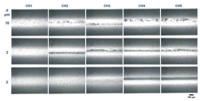
Fig. 4 Microscopy images of inert polystyrene particles in the microchannel at different positions (CH1-CH5) and for three different particle sizes. The particle concentration is  $0.63 \text{ g L}^{-1}$ , with an applied US voltage of 15 Vpp. The flow rate is  $0.1 \text{ ml min}^{-1}$ .
