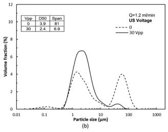
Fig. 10 Effect of US on the BaSO<sub>4</sub> particle size distribution at flow rates of (a) 0.8 ml min<sup>-1</sup> and (b) 1.2 ml min<sup>-1</sup>. The inserted tables show the average size  $(D_{50})$  and span  $(D_{90}-D_{10})$  of the distribution with and without US.
