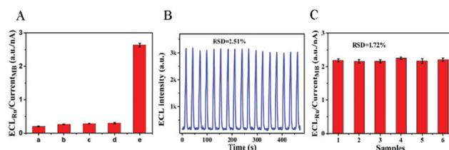
**Fig. 4** (A) Selectivity of the proposed biosensor after the incubation with (a) blank and 50 fM of (b) miRNA-499a, (c) miRNA-208b, (d) miRNA-328 and (e) miRNA-133a. (B) The ECL curves of the proposed ECL-EC ratiometric biosensor for detecting 400 aM miRNA-133a under 17 cycles of successive potential scans. (C) The repeatability of the constructed biosensor for detecting 10 fM miRNA-133a with six electrodes.
