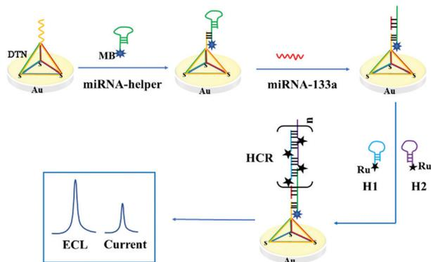
Scheme 1 Schematic illustration of the ECL-EC ratiometric biosensor.
