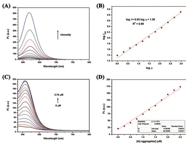
Fig. 1 (A) Solvent viscosity-dependent fluorescence changes of **Lyso-MC** (0.25  $\mu\text{M}$ ) in a water–glycerol system, (B) the linear relationship between  $\log I_{620}$  and  $\log \eta$  of **Lyso-MC**, (C) fluorescence spectroscopic titration of **Lyso-MC** (0.25  $\mu\text{M}$ ) towards  $A\beta_{1-42}$  aggregates in PBS buffer (pH = 7.4), (D) emission intensity of **Lyso-MC** as a function of the concentration of  $A\beta_{1-42}$  aggregates in PBS buffer (pH = 7.4).
