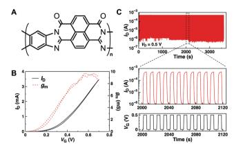
Fig. 4 (A) Chemical structure of BBL. (B) n-Type transfer curve (black) and transconductance (red dotted) of a 180 nm-thick BBL OECT measured at  $V_D$  = 0.6 V in 0.1 M NaCl. (C) Stability test of BBL OECT under sequential square wave gate voltage pulse for 1 h in water. Reprinted with permission from ref. 58 copyright The Authors.
