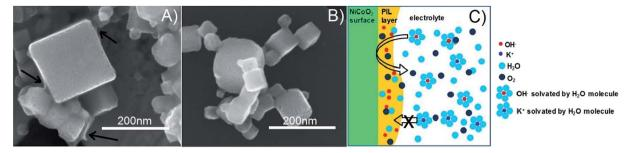
Fig. 6 (A) PIL covered  $NiCoO_2$  nanoparticles (arrows in black point at the edges of nanoparticles where the PIL is covering the catalyst), (B) PIL-free nanoparticles and (C) schematic illustration of the PEI. The PIL blocks metals at the electrode, while it is permeable to water, hydroxy ions and the as-generated oxygen, with bubbles nucleating outside the PEI layer.
