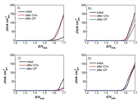
Fig. 3 Linear sweep voltammograms of a commercial mixed oxide NiCoO<sub>2</sub> catalyst with (A) PIL-1, (B) Nafion, (C) Fumion and (D) no binder from 1.2 to 1.7  $V_{RHE}$  with a sweep rate of 5 mV s<sup>-1</sup>, in 1 M KOH.
