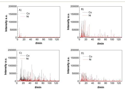
Fig. 5 ICP-OES transient profiles of a commercial mixed oxide NiCoO<sub>2</sub> with (A) PIL-1, (B) Nafion, (C) Fumion and (D) no binder in 1 M KOH. Corrosion profiles of each catalyst reveal a significantly better stability for the PIL-1 supported catalyst due to fast oxygen bubble removal from the catalyst surface.
