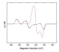
Fig. 7 Reversible binding of  $H_2$  by  $[1]^+[BAr_4^{F_4}]^-$  in the solid-state: CW X-band ESR spectra of powdered  $[1]^+[BAr_4^{F_4}]^-$  under Ar (black), followed by evacuation and subsequent admission of  $H_2$  (1 bar,  $[1\cdot H_2]^+[-BAr_4^{F_4}]^-$ , pink), and sequential evacuation to  $10^{-3}$  mbar and backfill with Ar (blue). All spectra recorded at 40 K.
