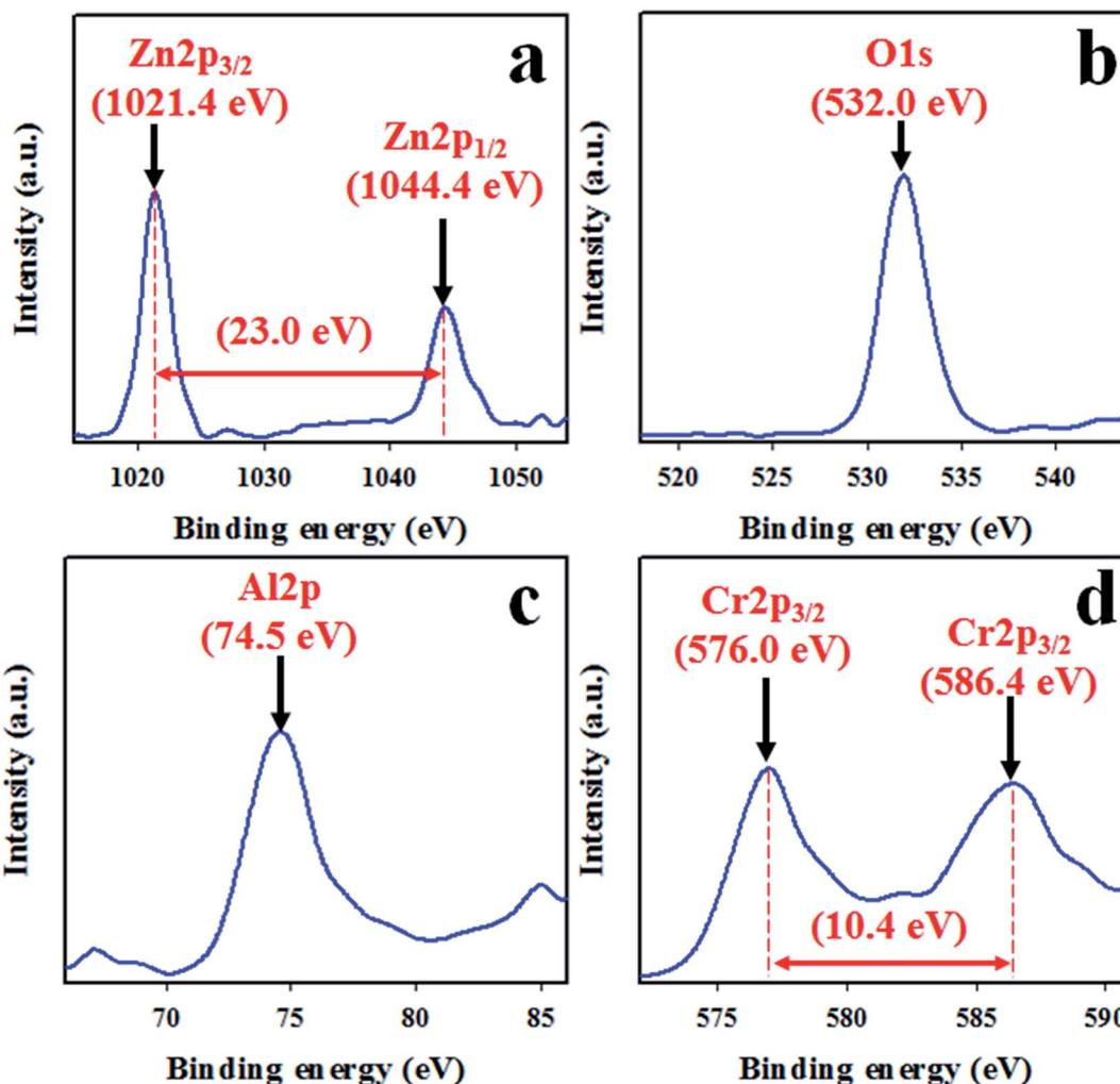
Fig. 2 High resolution XPS spectra of the  $\text{ZnO}/\text{Al}_2\text{O}_3/\text{Cr}_2\text{O}_3$  NPs. (a) The core level XPS spectrum of Zn 2p, (b) O 1s orbitals, (c) Al 2p orbitals, and (d) the 3/2 spin orbitals of Cr 2p.
