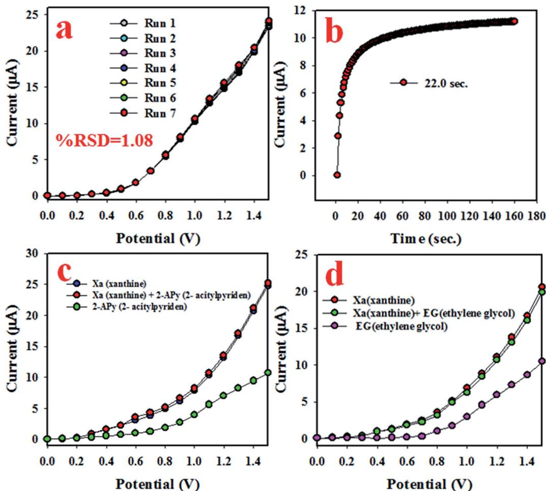
Fig. 5 Reliability investigations of the XNT sensor based on  $\text{ZnO}/\text{Al}_2\text{O}_3/\text{Cr}_2\text{O}_3$  NPs/binder/GCE: (a) testing reproducible performance, (b) response time, and (c and d) interference tests.
