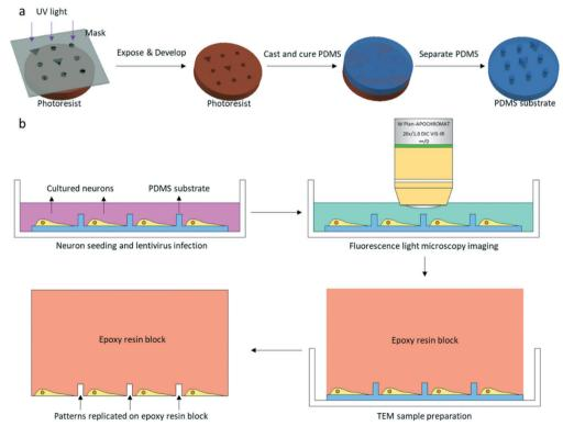
Fig. 1 Schematic of PDMS substrate fabrication, fluorescence light microscopy imaging, and transmission electron microscopy (TEM) sample preparation. (a) The conventional soft lithography method is used for PDMS substrate fabrication, and the patterns are custom-designed for FLM and EM correlation. (b) FLM imaging and TEM sample preparation. After FLM imaging, the TEM sample is prepared in the dish. Patterns designed on PDMS are replicated on the epoxy resin block.
