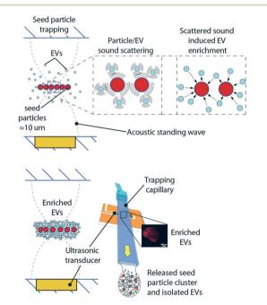
Fig. 10 Schematic of the acoustic trapping principle using acoustically trapped seed particles for EV enrichment. (top) EV enrichment by scattered sound interaction between seed particles (red) and EVs (light blue) (bottom) Enriched EV cluster washed from the plasma background in the acoustic trap and subsequently released in a droplet for biomarker analysis.
