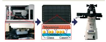
Fig. 1 Automated assay preparation and imaging. The assay is prepared by a pipetting robot (left) in a 384-well plate (center top). Each well contains a microtubule gliding assay where surfaceadsorbed kinesin-1 motors propel microtubules along the surface (center bottom). Movement of the fluorescently-labeled microtubules is recorded by a motorized inverted microscope (right).
