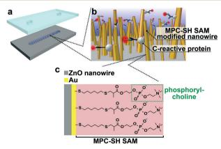
Fig. 1 (a) An illustration of MPC-SH SAM-modified nanowires in a microchannel. (b) An illustration of CRP recognition of MPC-SH SAMmodified nanowires. (c) Molecular formula of MPC-SH SAM on the Ausputtered nanowires. Phosphorylcholine groups specifically interact with CRP in the presence of calcium ions.
